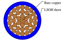
Bare copper conductor LSOH thermosetting insulation
